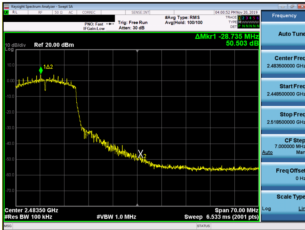
Plot 7-31. Band Edge Plot (802.11n (2.4GHz) – Ch. 10)
