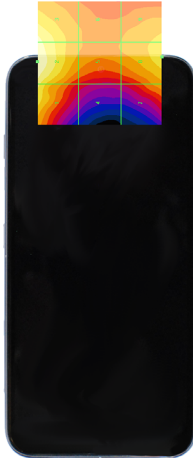
Figure 18-4 E-Field WD Scan overlay
