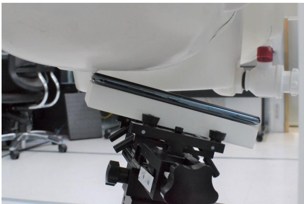
SAR Test Setup Photo 2 – Right Tilt
