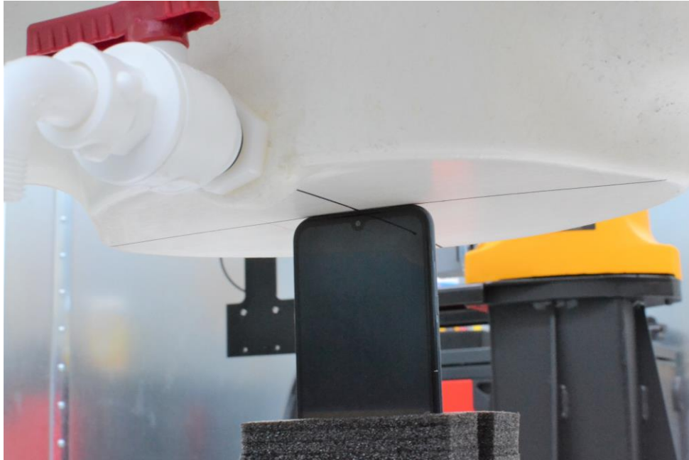
SAR Test Setup Photo 11 – Top Edge at 0 mm
