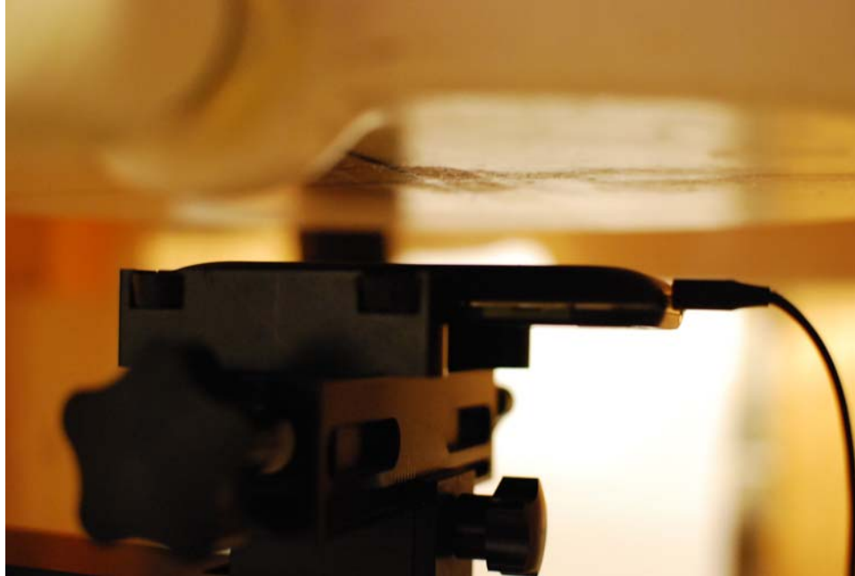
SAR Test Setup Photo 5: Body-Worn Back at 2.0 cm
