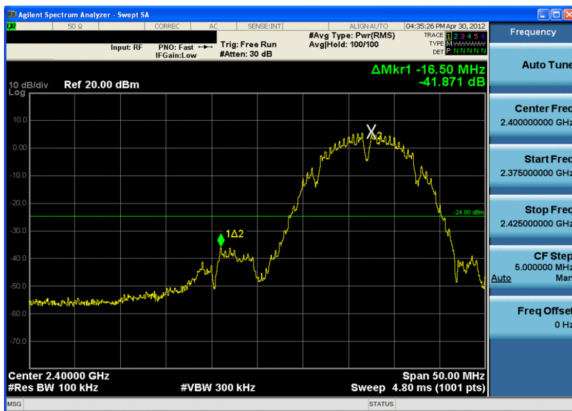
Plot 6-19. Band Edge Plot (802.11b – Ch. 1)
