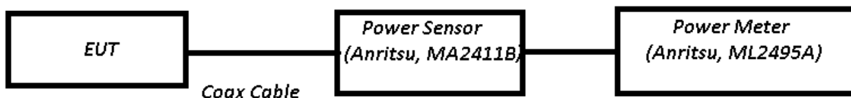
Figure 6-2. Test Instrument & Measurement Setup
