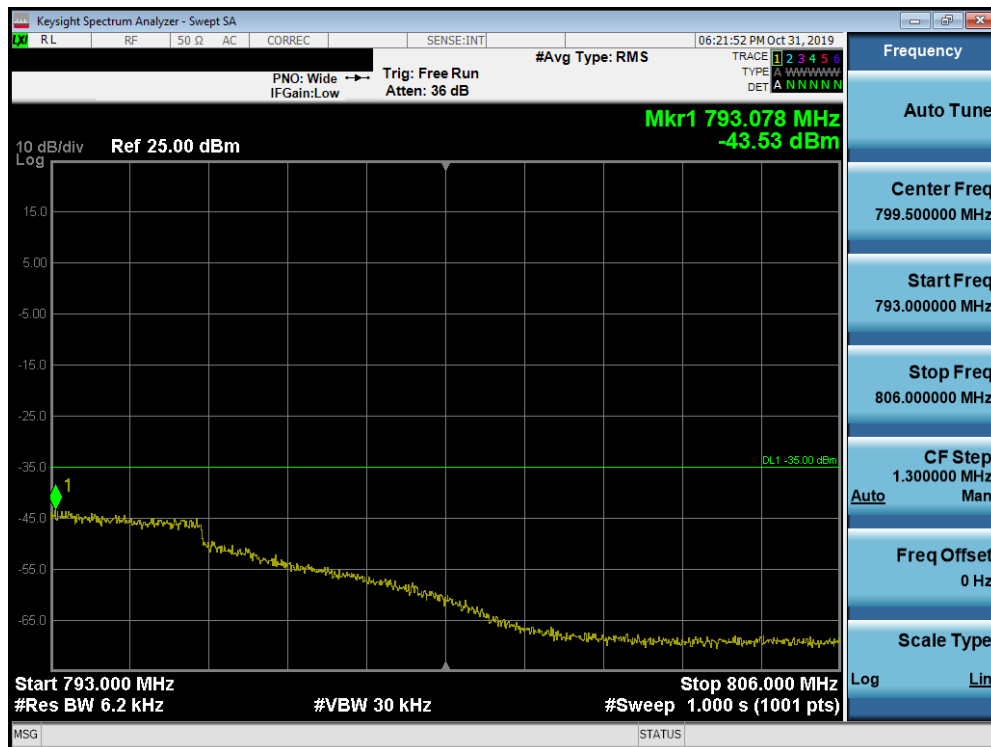
Plot 7-196. Upper Emission Mask Plot (Band 13 - 10.0MHz QPSK - Full RB Configuration)
