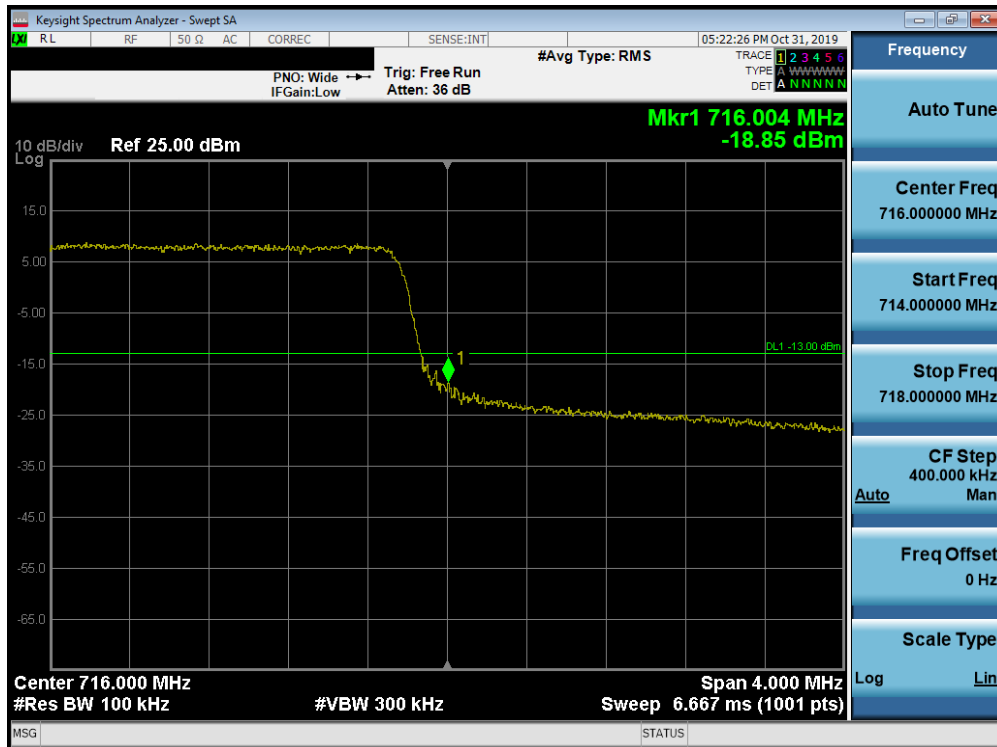
Plot 7-186. Upper Band Edge Plot (Band 12 - 5.0MHz QPSK - Full RB Configuration)
