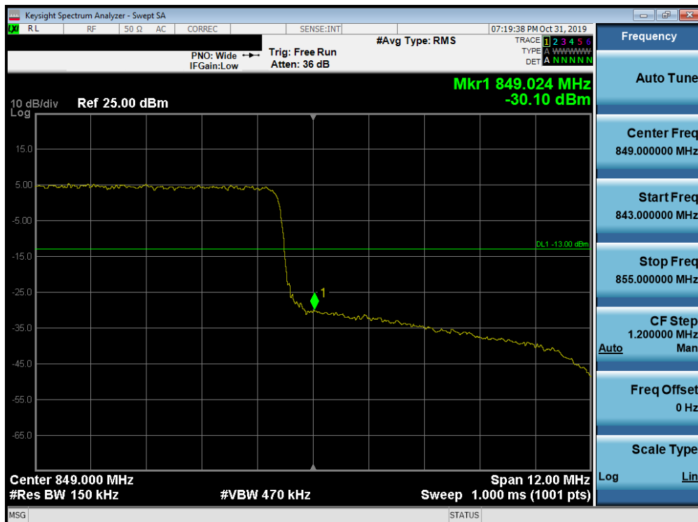
Plot 7-206. Upper Band Edge Plot (Band 26 - 15.0MHz QPSK - Full RB Configuration)
