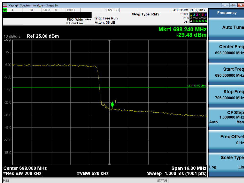
Plot 7-179. Upper Band Edge Plot (Band 71 - 20.0MHz QPSK - Full RB Configuration)
