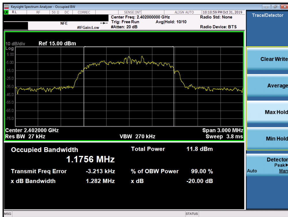
Plot 7-4. 20dB Bandwidth Plot (Bluetooth, 2Mbps – Ch. 0)
