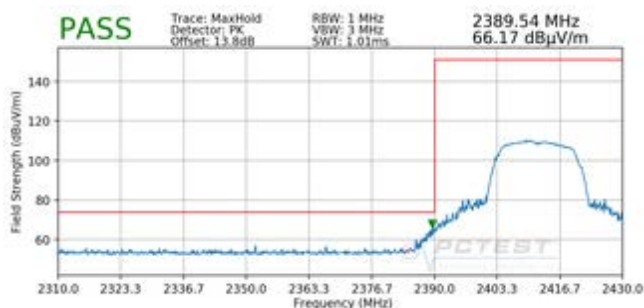
Plot 7-36. Radiated Restricted Lower Band Edge Measurement (Peak)
