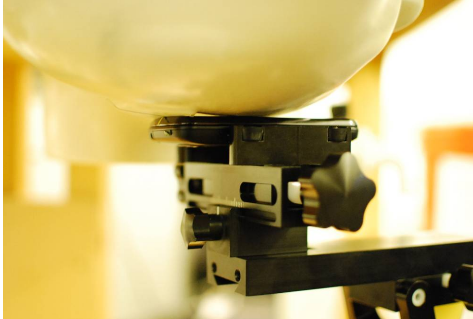
SAR Test Setup Photo 1 – Right Touch
