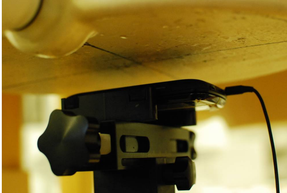
SAR Test Setup Photo 5 – Body-Worn at 2.0 cm
