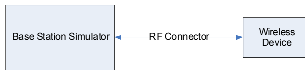
Figure 9-2 Power Measurement Setup
