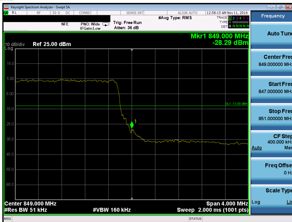
Plot 7-101. Upper Band Edge Plot (Band 5 - 5.0MHz QPSK - RB Size 25)
