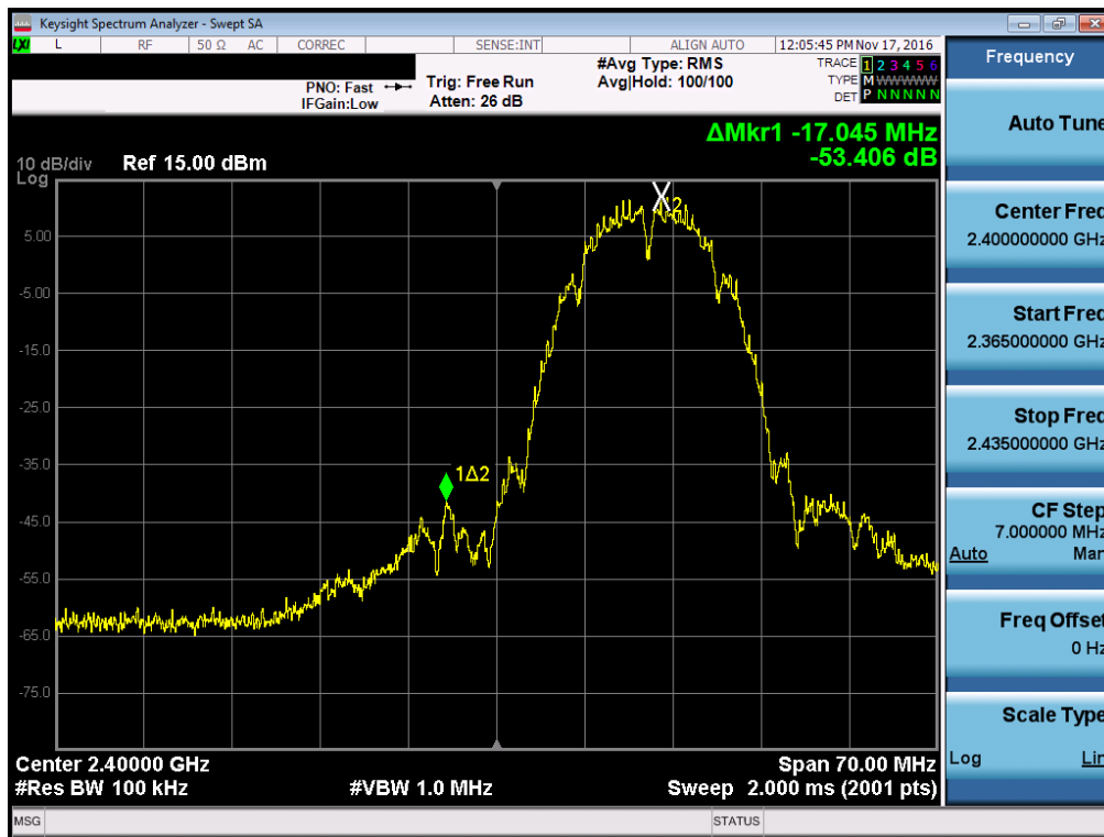
Plot 7-19. Band Edge Plot (802.11b – Ch. 1)
