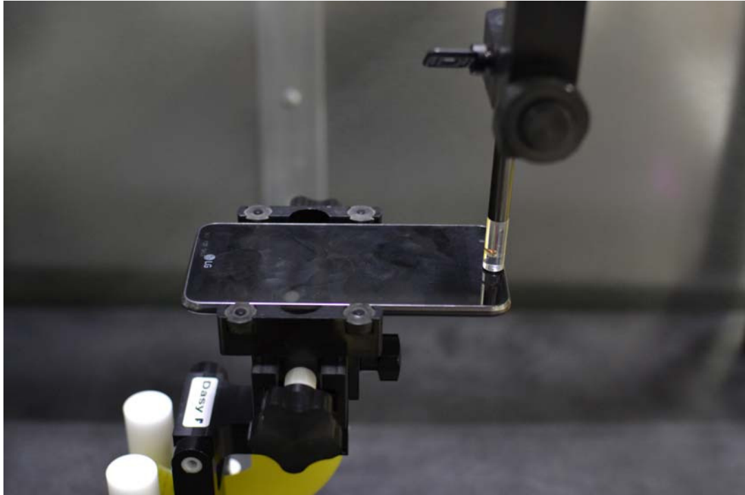
Figure 13-1 Test Setup for Wireless Device
