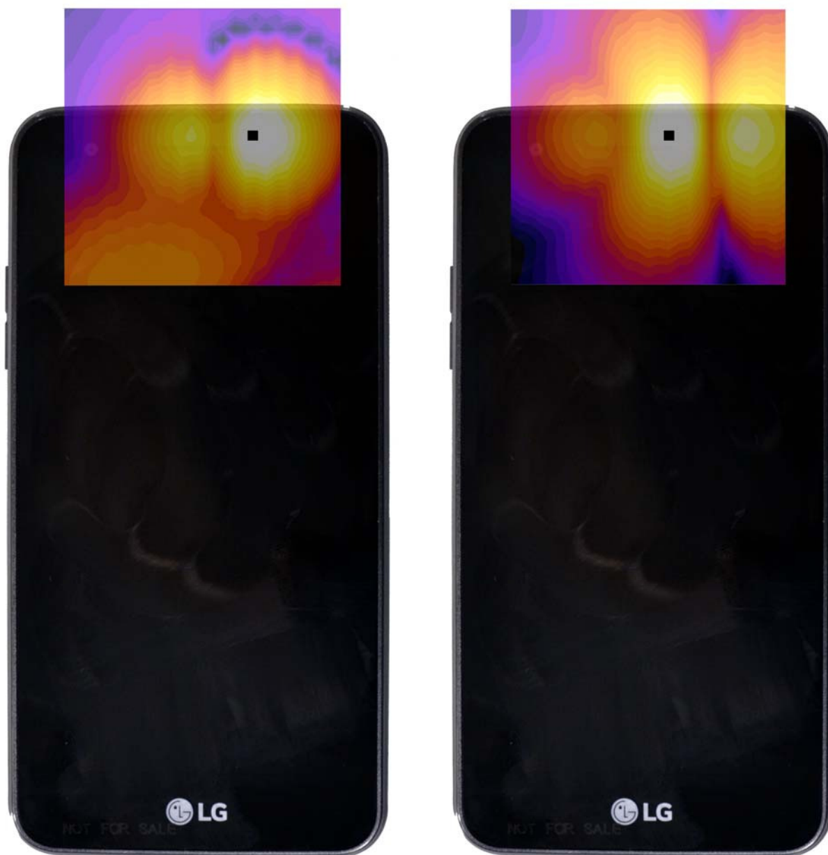
Figure 13-3 T-Coil Scan Overlay Magnetic Field Distributions
