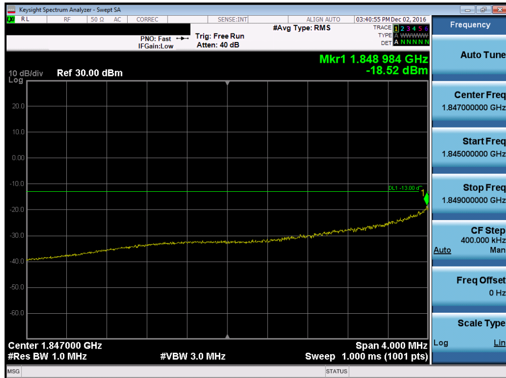
Plot 7-26. 4MHz Span Plot (PCS CDMA Mode – Ch. 25)
