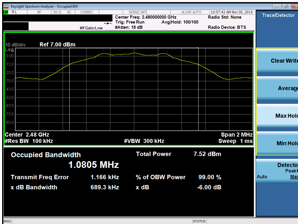
Plot 7-3. 6dB Bandwidth Plot (Bluetooth (LE) – Ch. 39)
