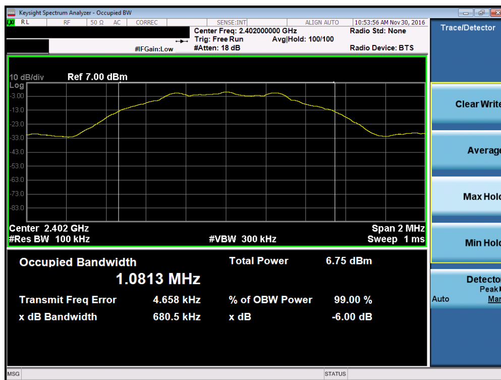
Plot 7-1. 6dB Bandwidth Plot (Bluetooth (LE) – Ch. 0)
