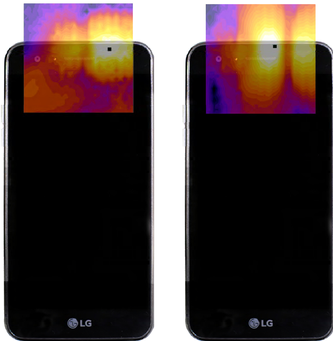
Figure 13-3 T-Coil Scan Overlay Magnetic Field Distributions
