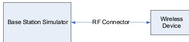
Figure 9-2 Power Measurement Setup
