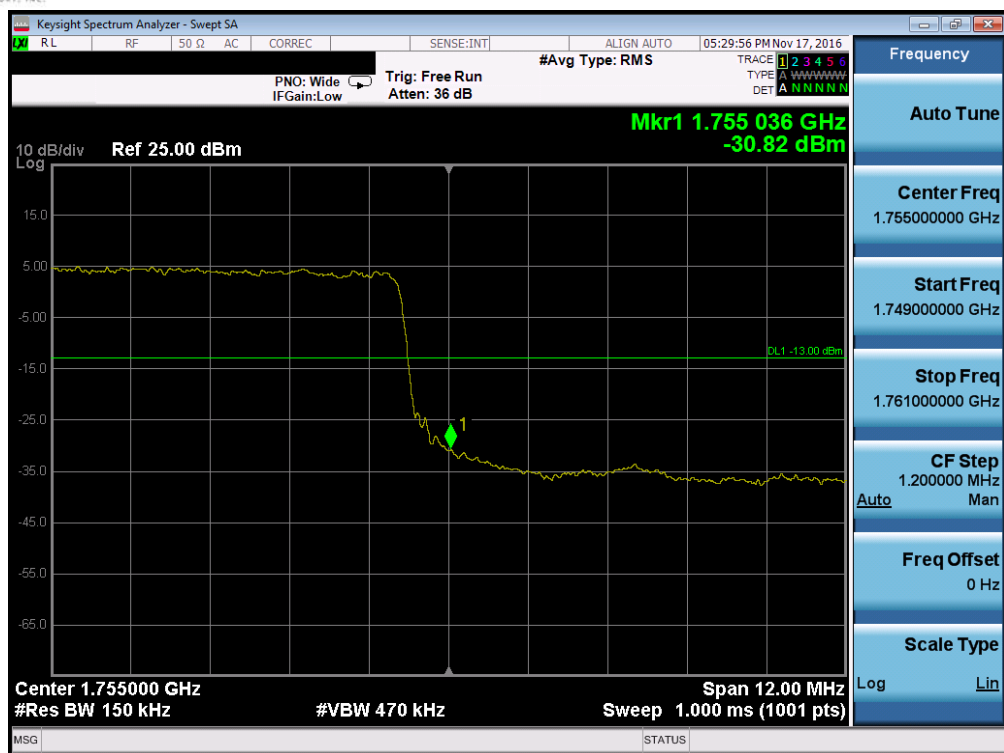
Plot 7-123. Upper Band Edge Plot (Band 4 – 15.0MHz QPSK – RB Size 75)
