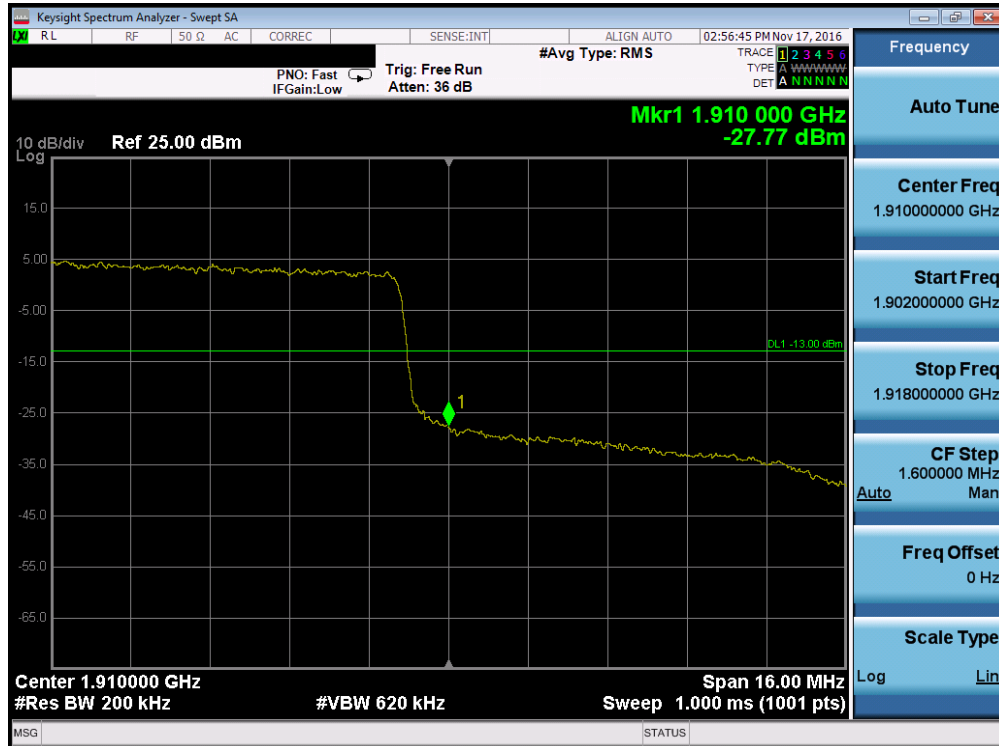
Plot 7-151. Upper Band Edge Plot (Band 2 – 20.0MHz QPSK – RB Size 100)
