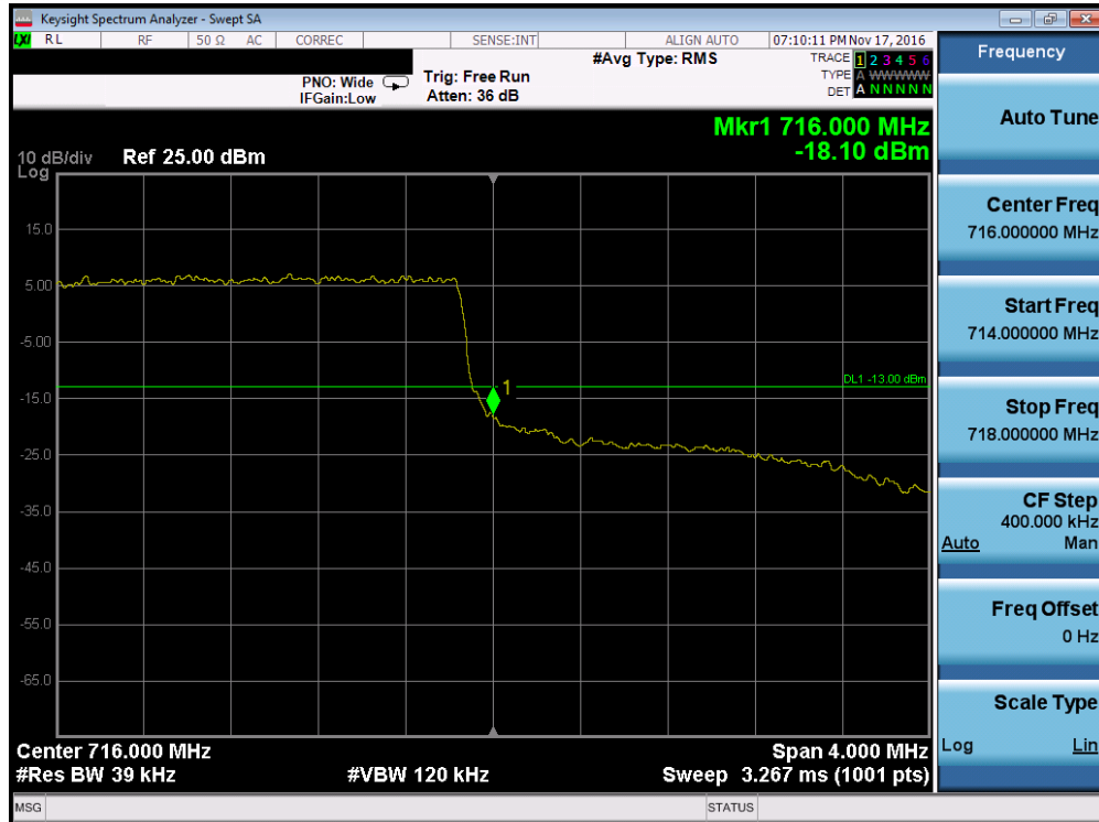
Plot 7-83. Lower Band Edge Plot (Band 12 – 3.0MHz QPSK – RB Size 15)
