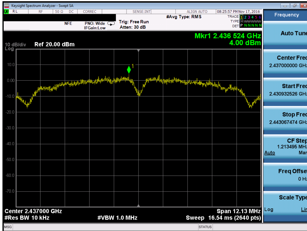
Plot 7-11. Power Spectral Density Plot (802.11b – Ch. 6)
