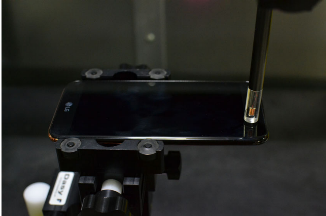
Figure 13-1 Test Setup for Wireless Device
