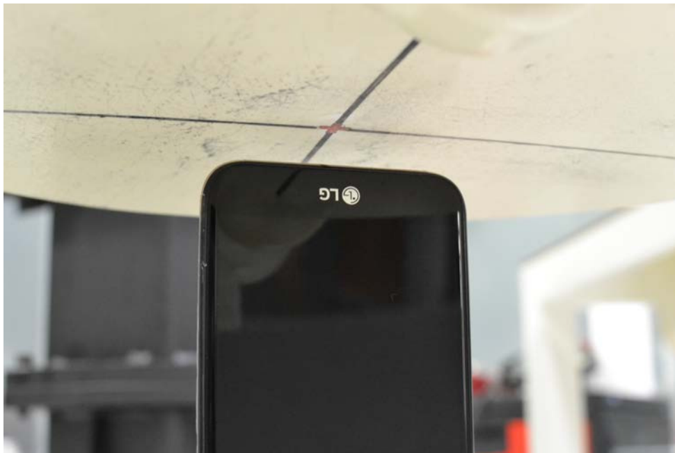
SAR Test Setup Photo 8 – Bottom Edge at 1.0 cm
