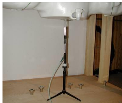
Figure 10-2 System Verification Setup Photo
