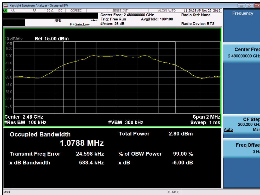
Plot 7-3. 6dB Bandwidth Plot (Bluetooth (LE) – Ch. 39)
