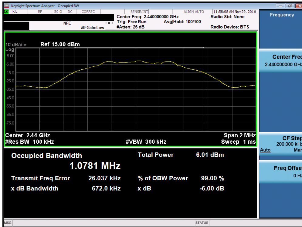
Plot 7-2. 6dB Bandwidth Plot (Bluetooth (LE) – Ch. 19)
