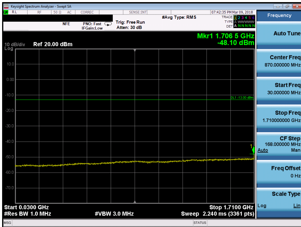
Plot 7-121. Conducted Spurious Plot (Band 66/4 - 20.0MHz QPSK - RB Size 1, RB Offset 0 - Mid Channel)
