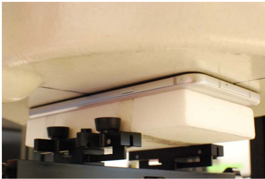
SAR Test Setup Photo 8 – Front Side at 0 mm
