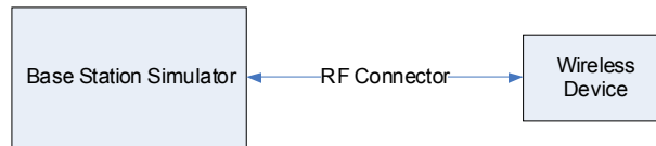
Figure 9-1 Power Measurement Setup
