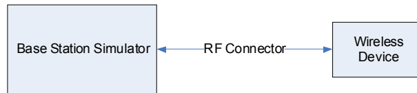
Figure 9-2 Power Measurement Setup
