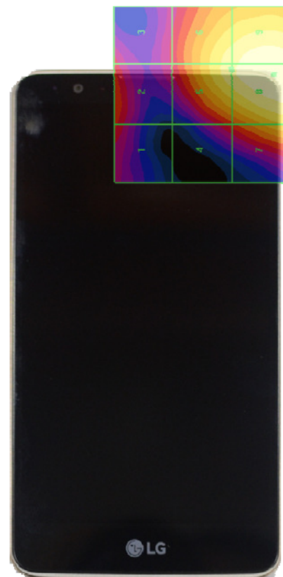
Figure 18-4 E-Field WD Scan overlay (T-coil centered scan area pictured)
