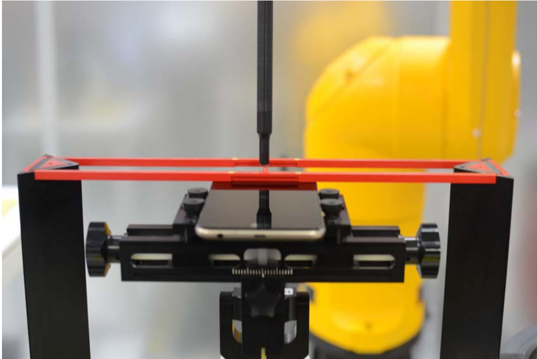
Figure 18-1 Ear Reference Point HAC Phantom Alignment
