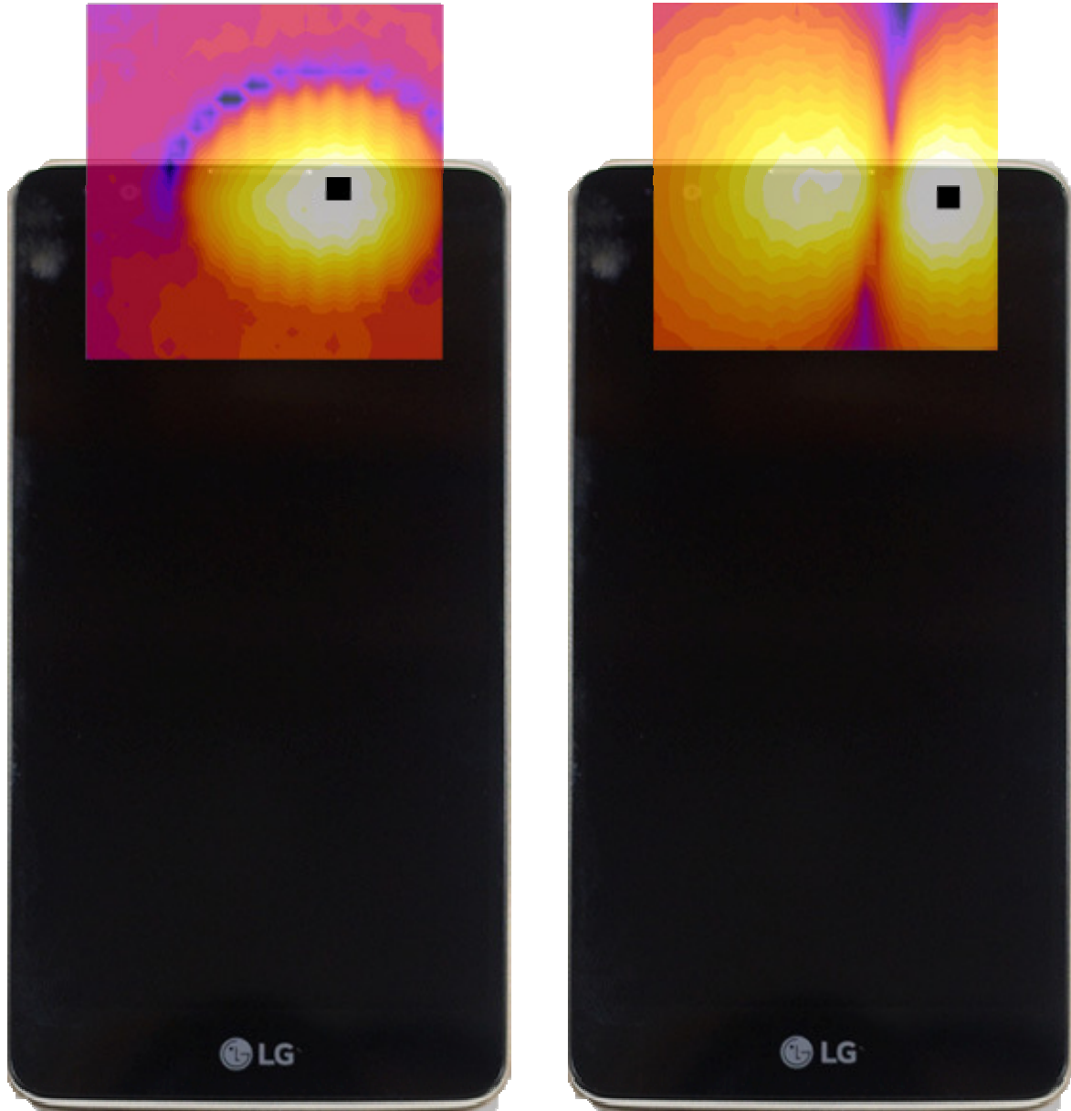
Figure 14-3 T-Coil Scan Overlay Magnetic Field Distributions
