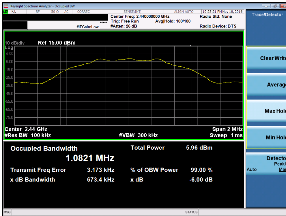
Plot 7-2. 6dB Bandwidth Plot (Bluetooth (LE) – Ch. 19)
