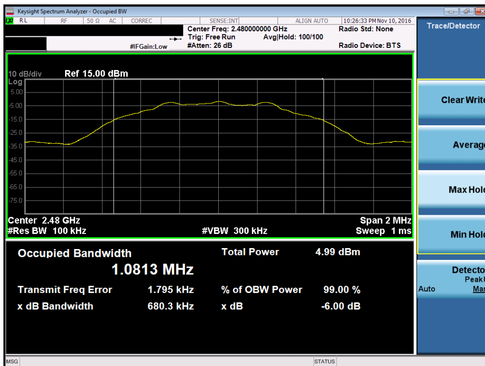
Plot 7-3. 6dB Bandwidth Plot (Bluetooth (LE) – Ch. 39)
