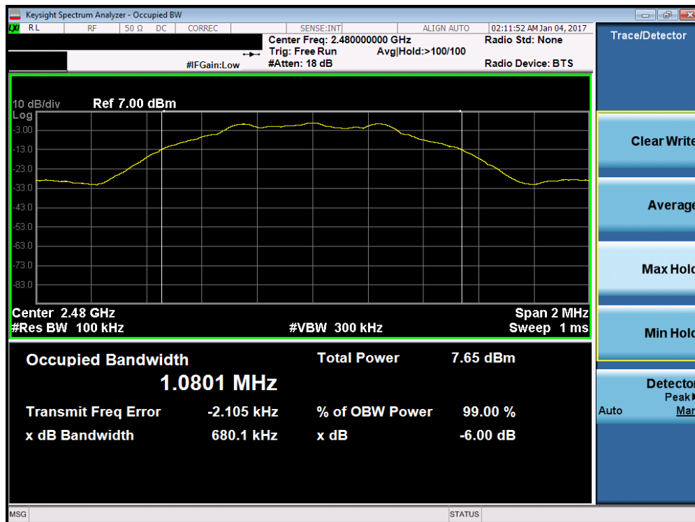
Plot 7-3. 6dB Bandwidth Plot (Bluetooth (LE) – Ch. 39)
