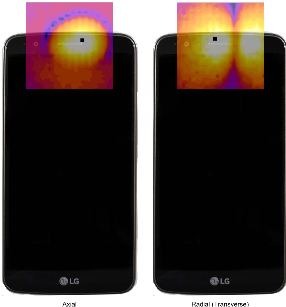
Figure 13-3 T-Coil Scan Overlay Magnetic Field Distributions
