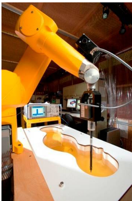
Figure 3-2 SAR Measurement System
