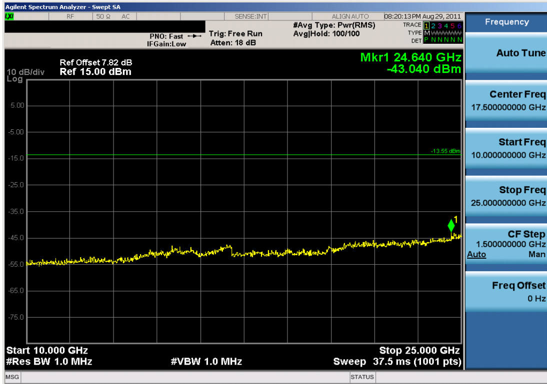
Plot 6-19. Conducted Spurious Plot (Bluetooth, 2Mbps – Ch. 0)
