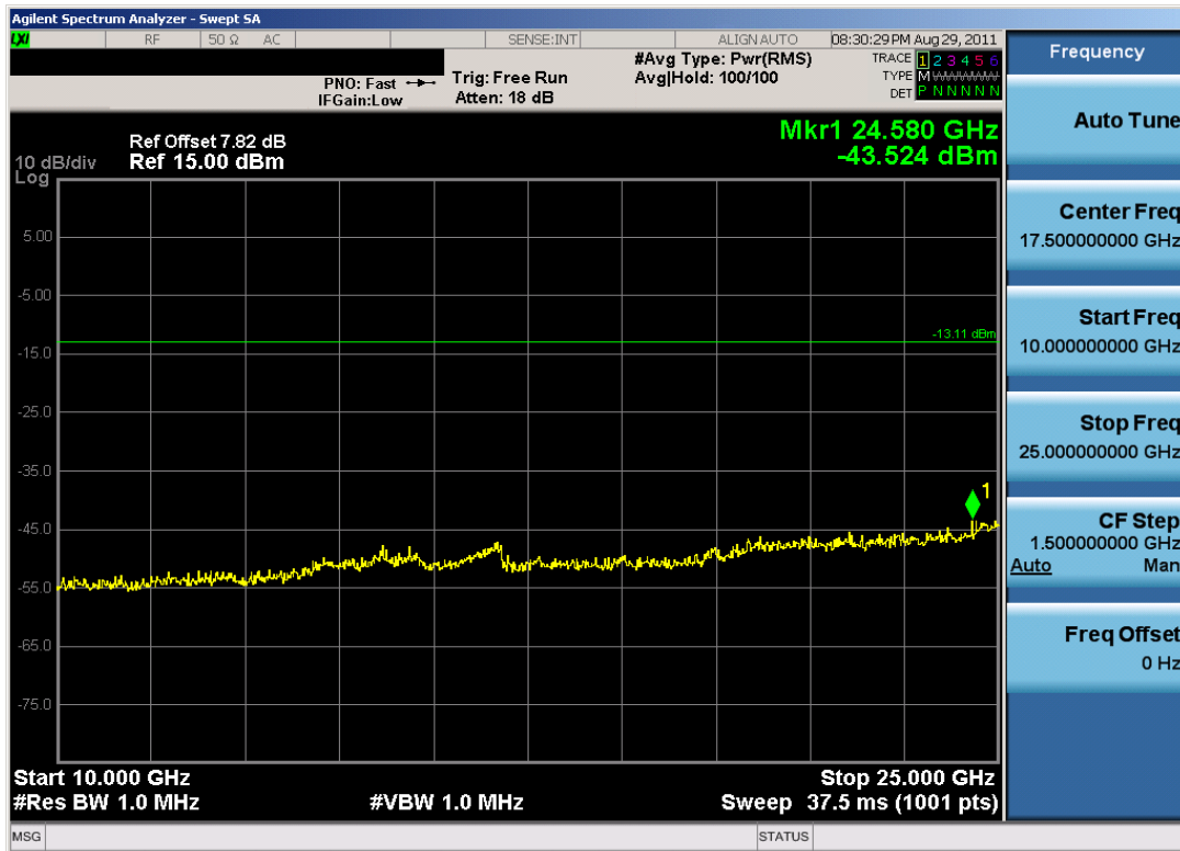
Plot 6-21. Conducted Spurious Plot (Bluetooth, 2Mbps – Ch. 39)
