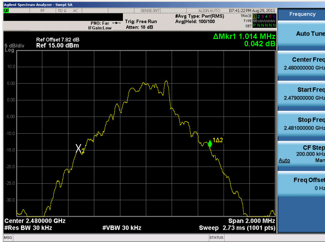
Plot 6-3. 20dB Bandwidth Plot (Bluetooth, 1Mbps – Ch. 78)
