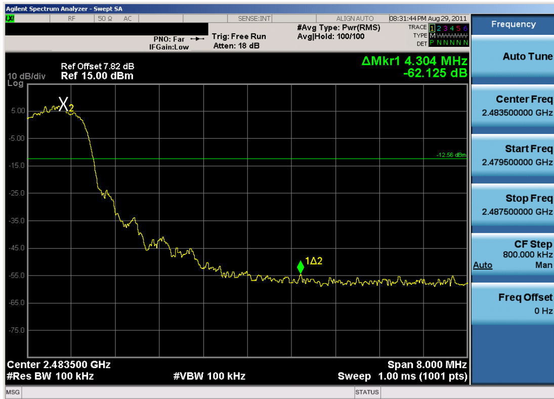
Plot 6-13. Band Edge Plot (Bluetooth, 2Mbps - Ch. 78)
