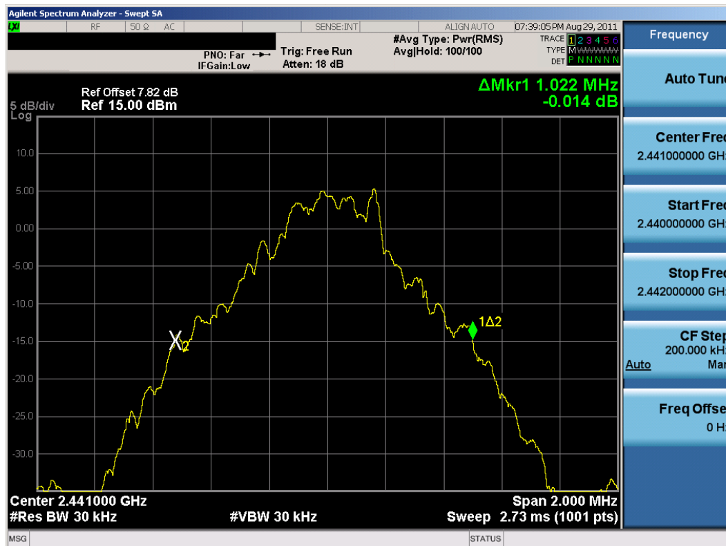
Plot 6-2. 20dB Bandwidth Plot (Bluetooth, 1Mbps – Ch. 39)
