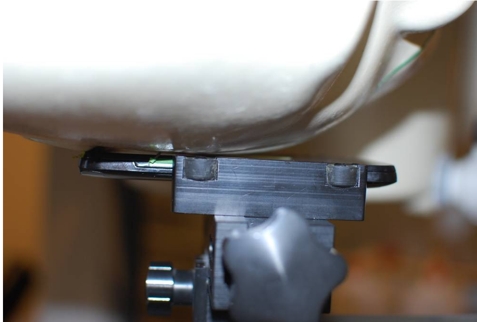
SAR Test Setup Photo 1 – Right Touch
