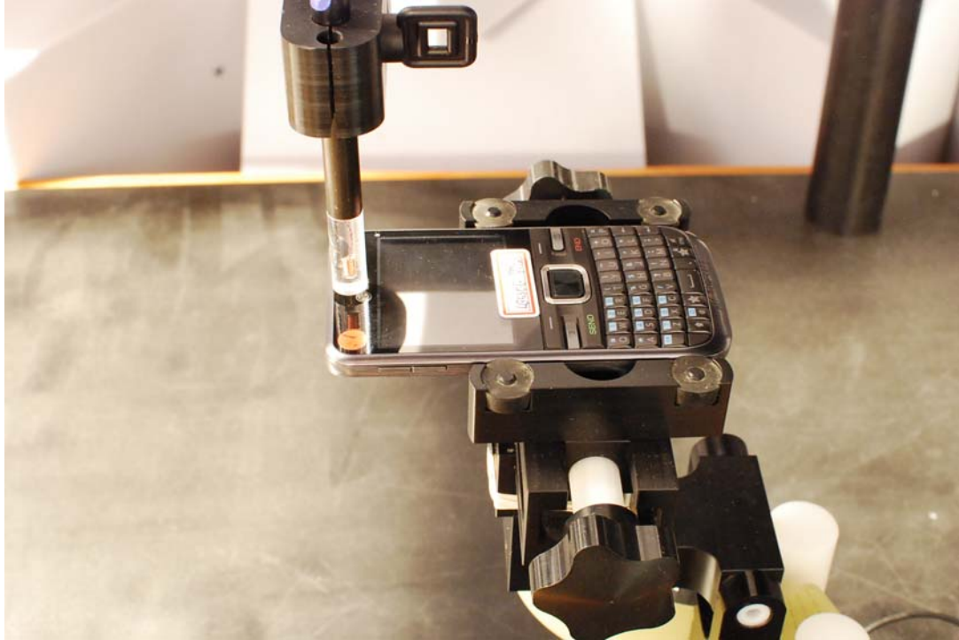
Figure 13-1 Test Setup for Wireless Device
