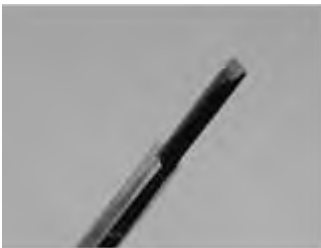
Figure 4.4 EX3DV4 E-field Probe
