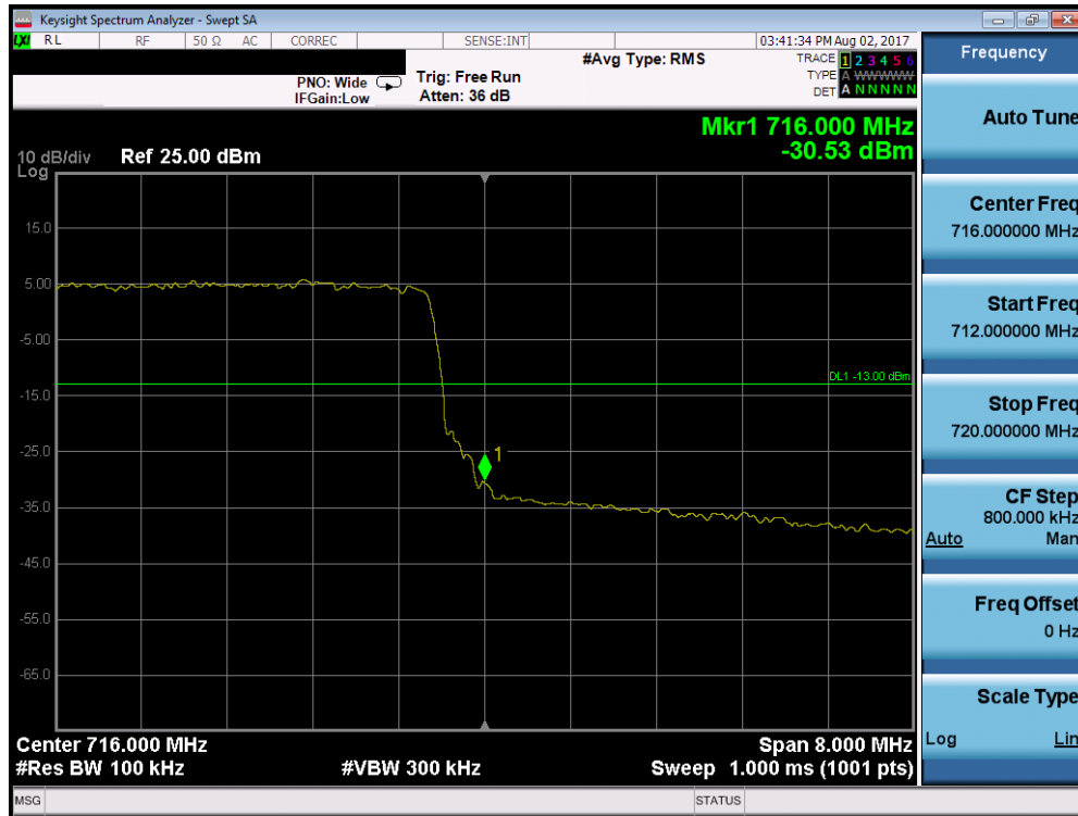
Plot 7-103. Upper Band Edge Plot (Band 12 – 10.0MHz QPSK – RB Size 50)
