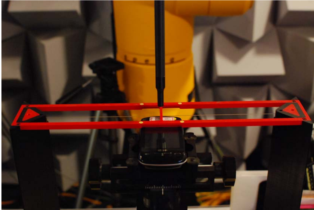
Figure 17-1 Ear Reference Point HAC Phantom Alignment
