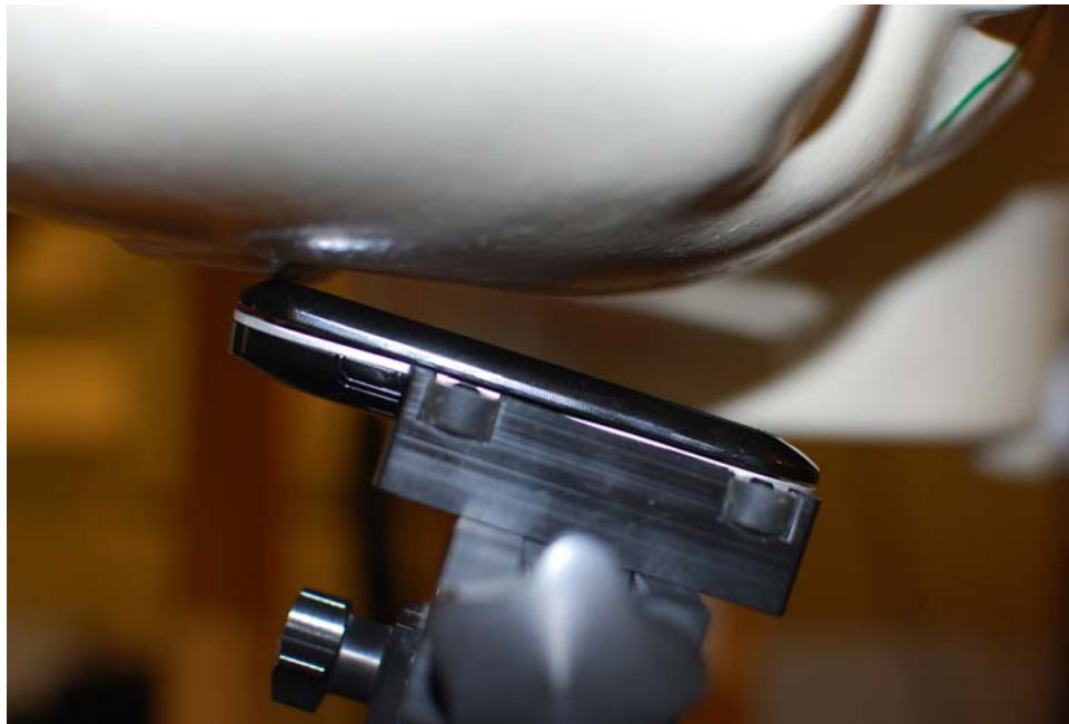
SAR Test Setup Photo 2: Right Tilt
