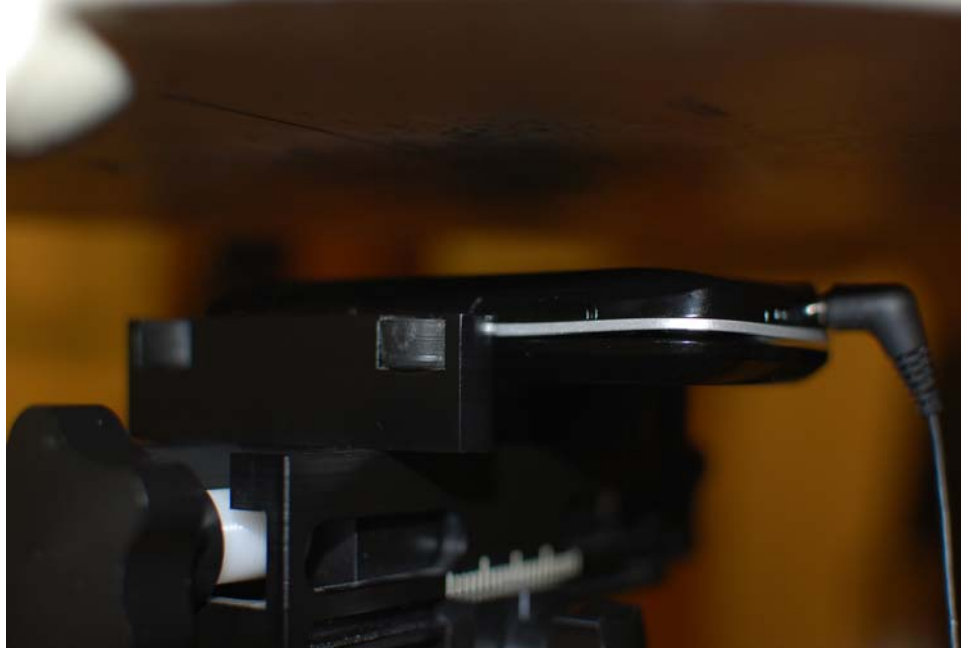
SAR Test Setup Photo 5: Body-Worn at 2.0 cm
