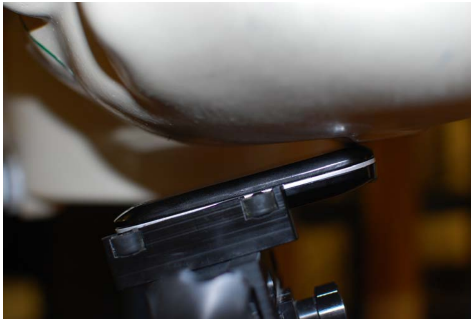
SAR Test Setup Photo 4: Left Tilt
