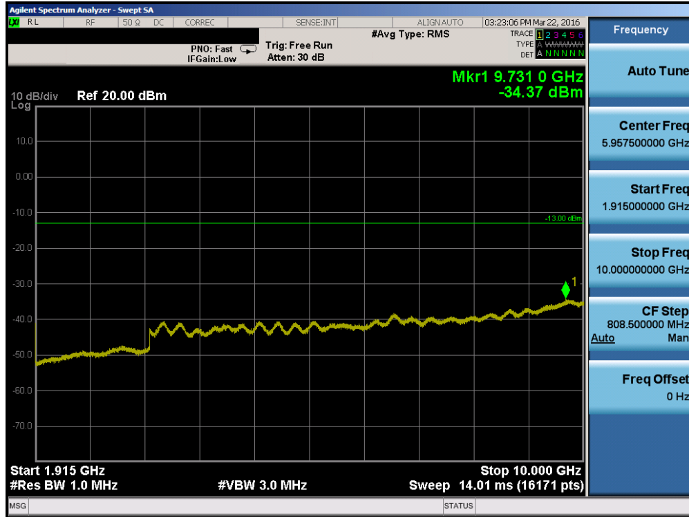
Plot 7-44. Conducted Spurious Plot (PCS CDMA Mode – Ch. 1175)
