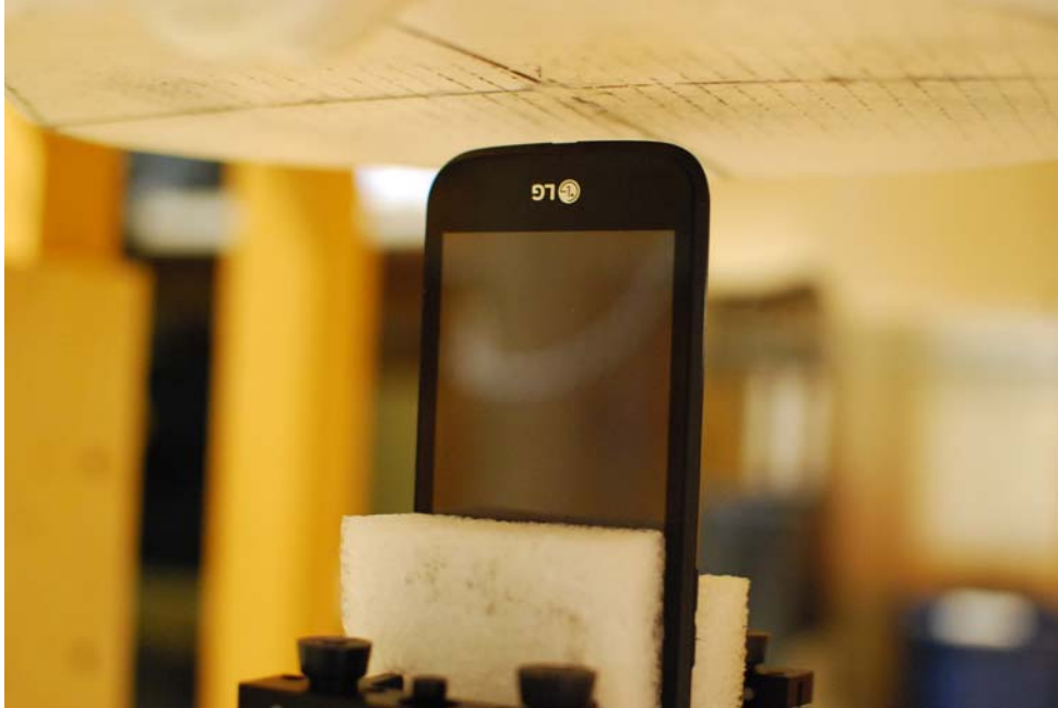
SAR Test Setup Photo 8 – Bottom at 1.0 cm
