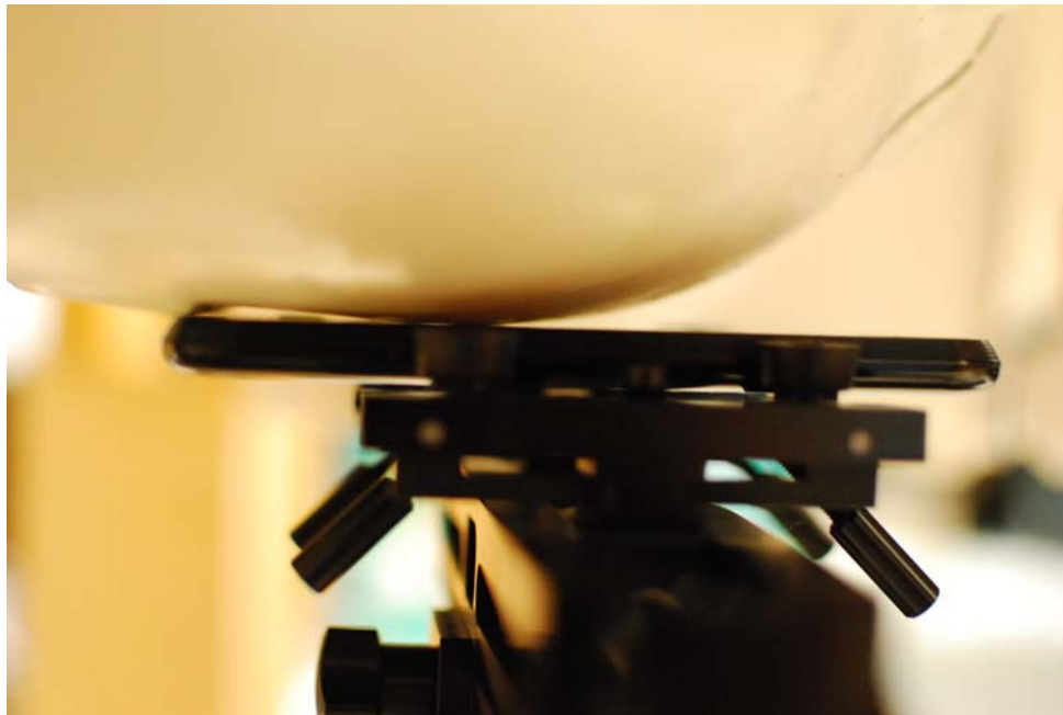
SAR Test Setup Photo 1 – Right Cheek
