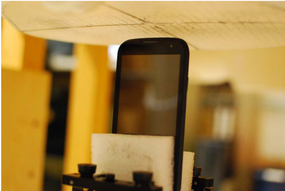
SAR Test Setup Photo 7: top at 1.0 cm
