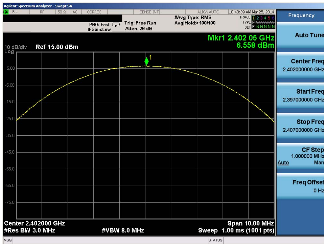
Plot 6-13. Peak Conducted Power (2Mbps – Ch. 0)
