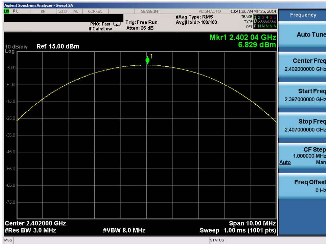
Plot 6-16. Peak Conducted Power (3Mbps – Ch. 0)
