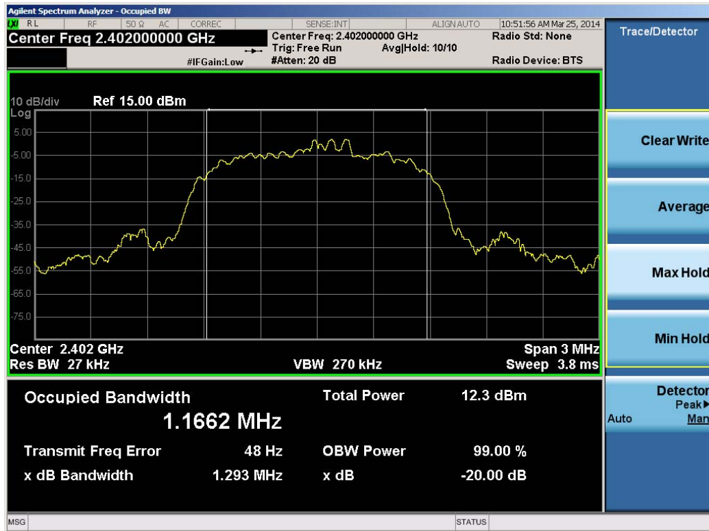
Plot 6-7. 20dB Bandwidth Plot (Bluetooth, 3Mbps – Ch. 0)
