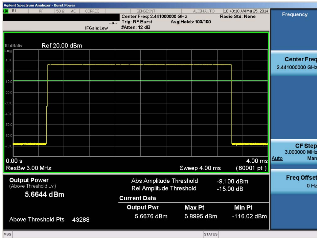
Plot 6-20. Average Conducted Power (1Mbps – Ch. 39)
