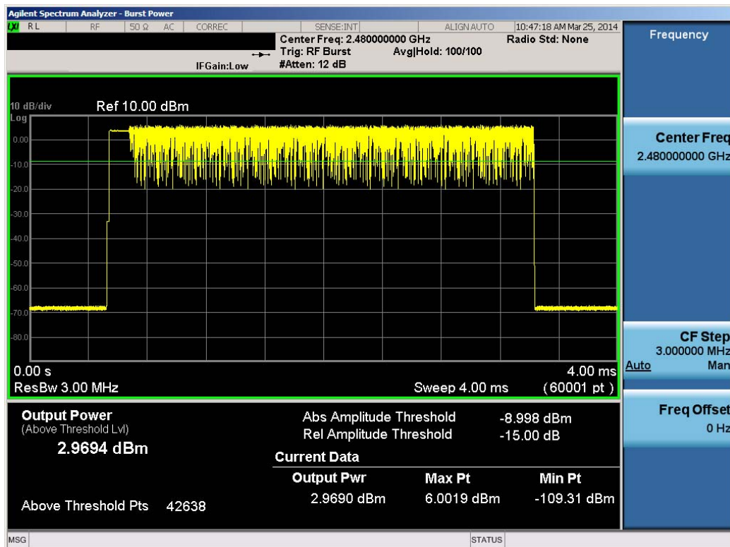
Plot 6-27. Average Conducted Power (3Mbps – Ch. 78)
