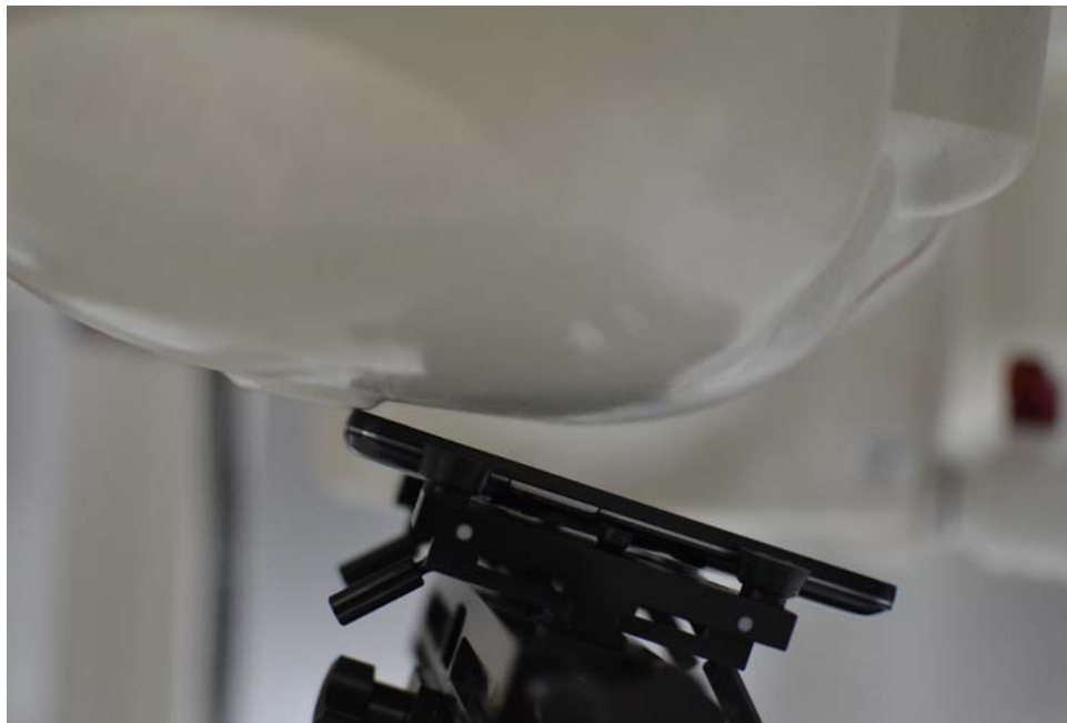
SAR Test Setup Photo 2- Right Tilt
