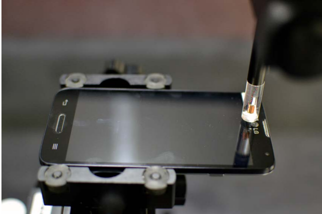
Figure 13-1 Test Setup for Wireless Device
