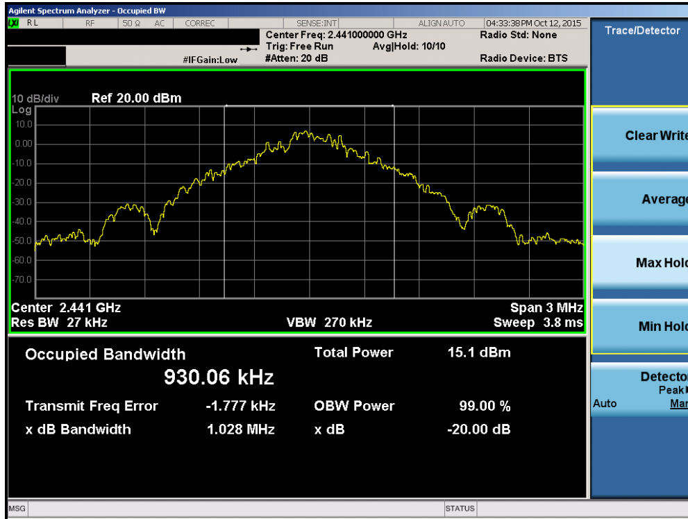
Plot 7-2. 20dB Bandwidth Plot (Bluetooth, 1Mbps – Ch. 39)
