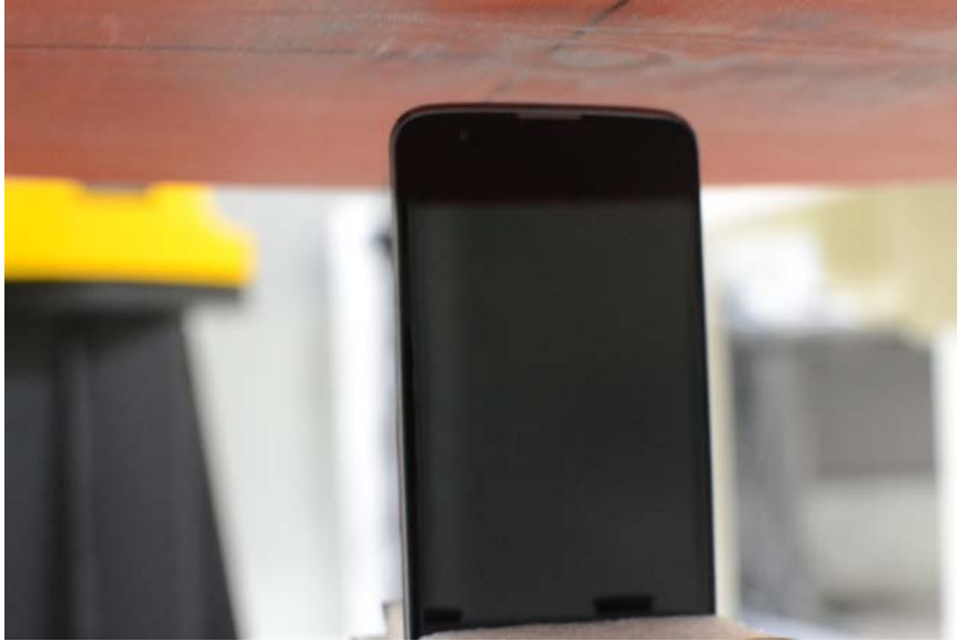
SAR Test Setup Photo 7 – Top Edge (10 mm)
