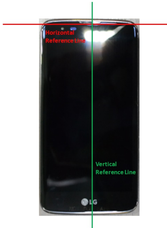
SAR Test Setup Photo 11 – Horizontal and Vertical Reference Lines
