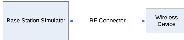
Figure 9-3 Power Measurement Setup
