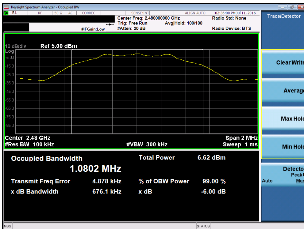
Plot 7-3. 6dB Bandwidth Plot (Bluetooth (LE) – Ch. 39)
